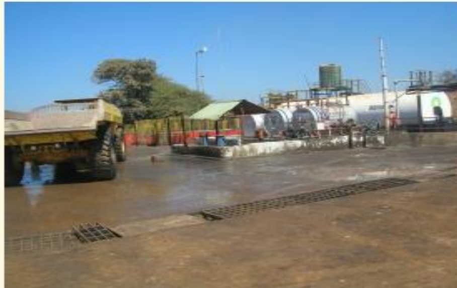
Spilled oil comingling with water from the Mine wash bay and eventually to the environment -Chibuluma Mining Plc
